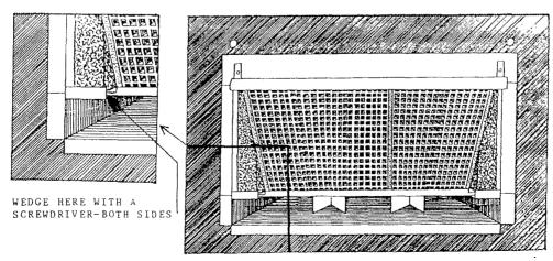
REPLACEMENT: Replace the catalytic combustor with NHC, Inc. part number 5100-2292. The combustor has been designed for many thousands of hours of use. The combustor should be replaced when any of the following symptoms occur:
