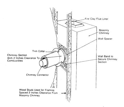
THIMBLE: A thimble must be used when the connection from the stove is made through a combustible wall to a masonry chimney. There are several methods to use the connection through a combustible wall. Local building authorities may be consulted or NFPA 211 may be used for referencing methods of chimney connection.
