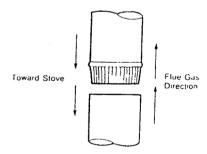
Additional stovepipe accessories (draw-bands, slip-joints, clean-out tees) greatly simplify the connection of stovepipe to chimney, make inspection easier, and let you dismantle the stovepipe without moving the stove. Because the Harvest comes equipped with a stove pipe damper in the flue collar, an additional damper in the stove pipe is not necessary.
