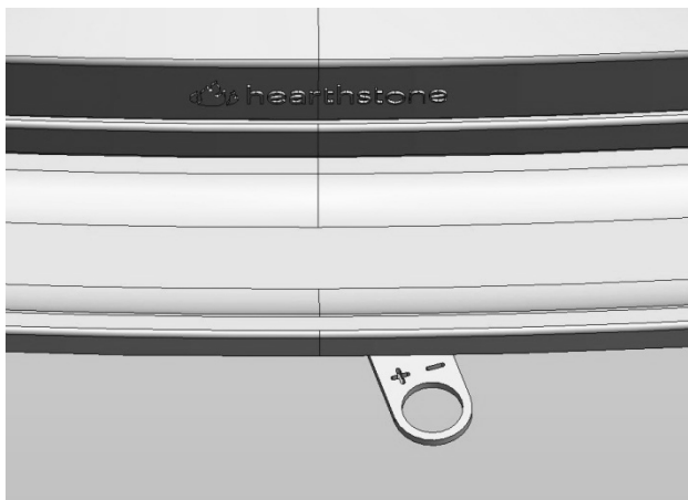
Figure 13 – Air Control Low Position
