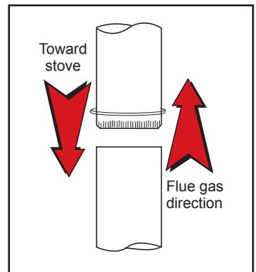
Figure 5.3 - Chimney connector.
