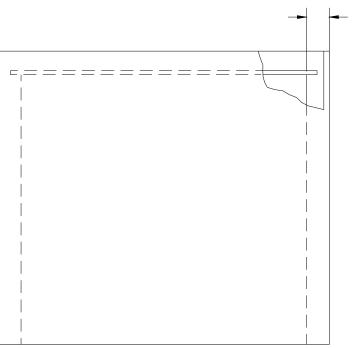
2. Attach the heat shield to the stove using the screws provided. Place the spacer between the heat shield and the stove back. The screw will go through the spacer.
