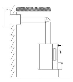
FIGURE 9 - INSTALLATION INTO A FACTORY BUILT CHIMNEY
