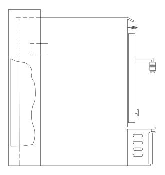
FIGURE 12 INSTALLING THE HEAT SHIELD
