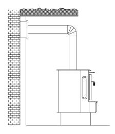
FIGURE 8 - INSTALLATION INTO A MASONRY FLUE
