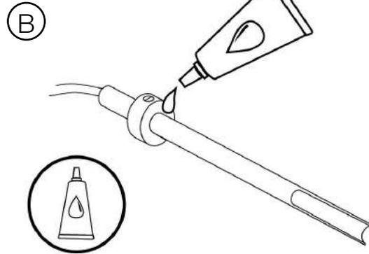
Liberally spread stove cement (not supplied) along the bottom of depth gauge.
