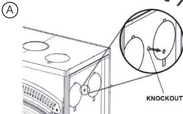
Remove the knockout tab.
