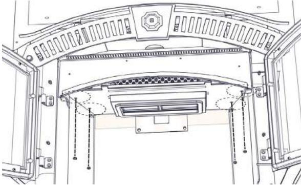
Remove nuts & bolts on either side of appliance while supporting the baffle.
