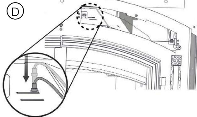
Slide the straightened probe into the hole.
