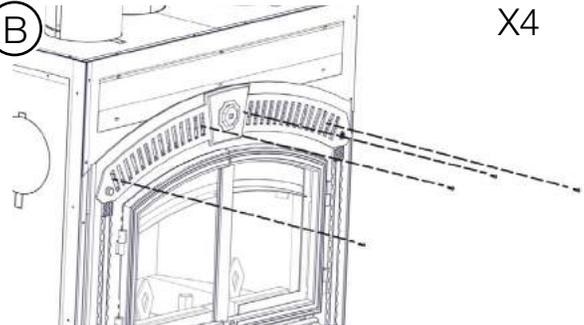
Unscrew the four retaining screws.
