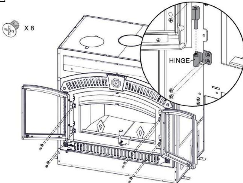
Install hinges to firebox front, using screws provided.
