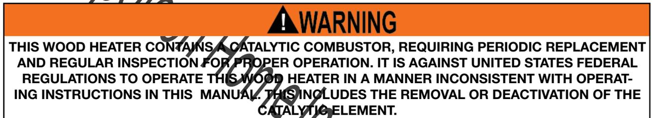
Periodic inspection of the catalytic combustor is needed to ensure proper functioning of the unit and also to determine when replacement is required. Creosote buildup, increase in emissions and a loss of heat efficiency will result from a non-functioning combustor unit.
