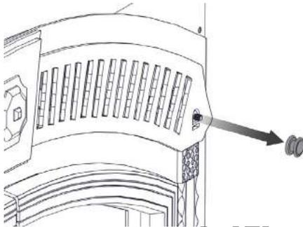
Loosen set screw, unthread and remove the knob on the right side of the decorative trim.
