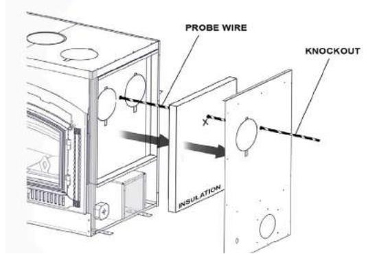
Removing side panels is not necessary. The diagram above is for illustrative purposes only.
