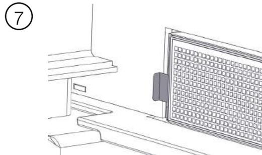
Grab the steel tabs located on either side of the catalyst.
