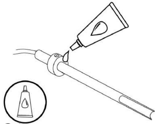
Liberaly spread stove cement (not supplied) along the bottom of depth gauge.
