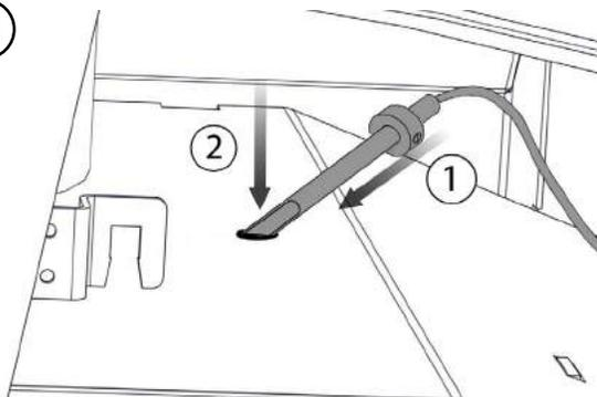
Insert the probe on an angle and gradually straighten the probe so that it aims down.
