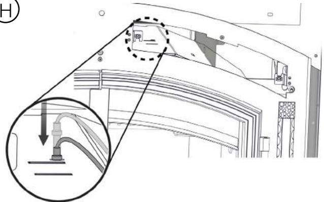
Slide the straightened probe into the hole.
