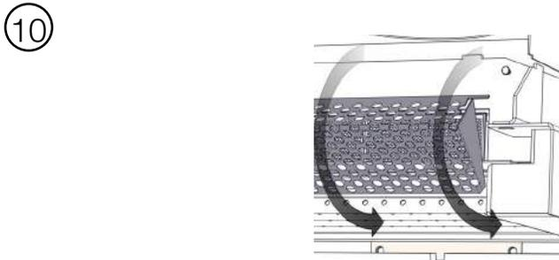
Reinstall perforated catalyst shield in reverse.
