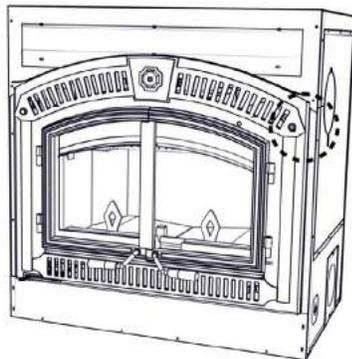
Ensure bypass door is open during start up and refueling. See above for bypass door rod location.
