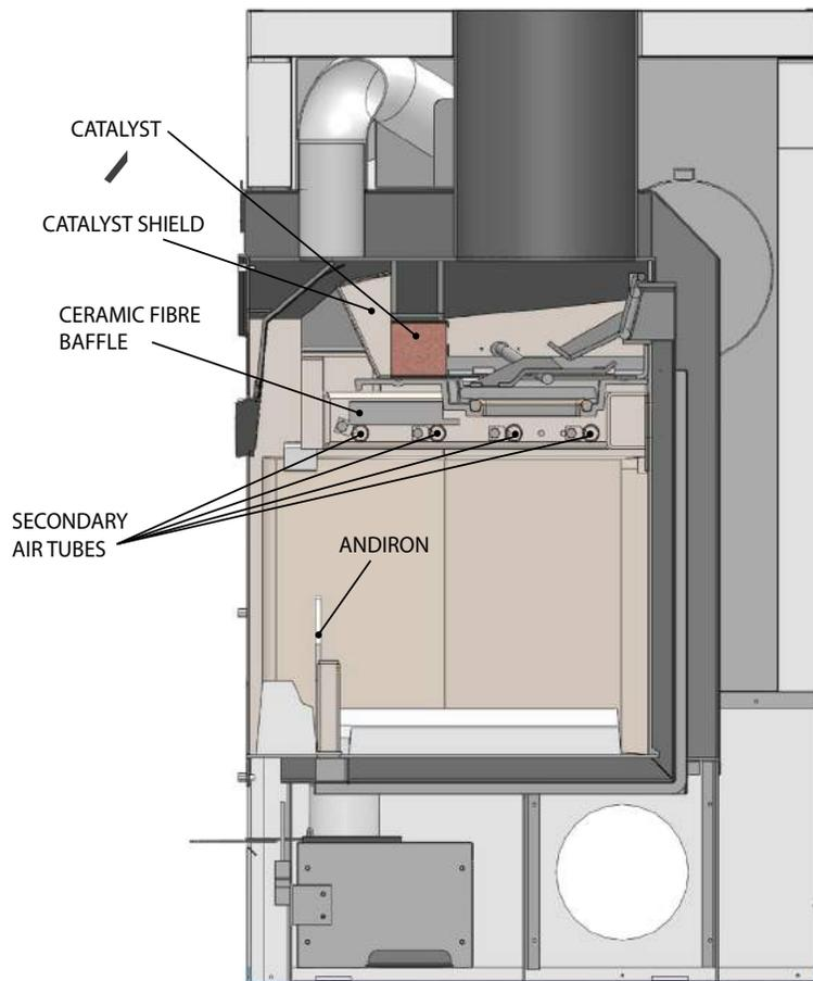
The NZ3000H contains a ceramic fibre baffle, catalyst and catalyst shield. It is important that each of these components are installed correctly prior to operating the unit.
