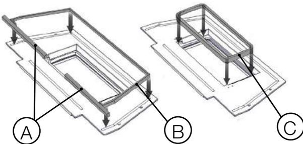
Replace gaskets A ,B and C. Secure with stove cement (not supplied).
