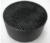
*<br>Creosote | Excess build up of Creosote or Fly-Ash                          | - Clean plugged cells<br>- Burn only dry seasoned wood<br>- Engage catalyst only when light-off temperatures are met      |
