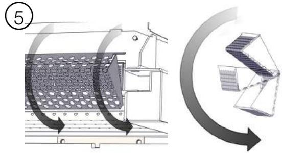
Pivot the perforated catalyst shield forwards until it is facing downwards .
