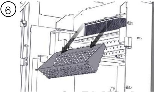
Remove perforated catalyst shield.
