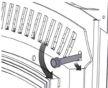
Press bypass rod downwards then inwards to lock into place.
