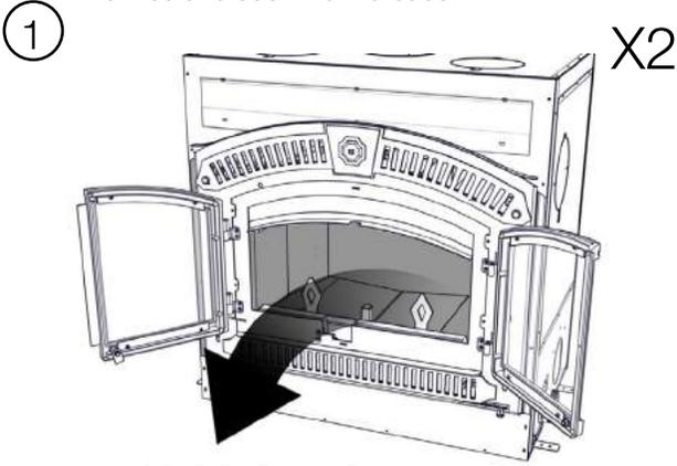
Remove all the bricks panels inside of the appliance. See STEP 2 for brick removal order.
