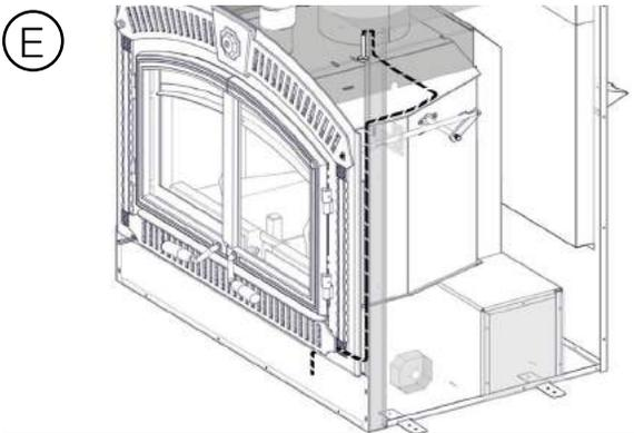
OPTION 1 . This option allows the wire to exit directly through the bottom trim grill.
