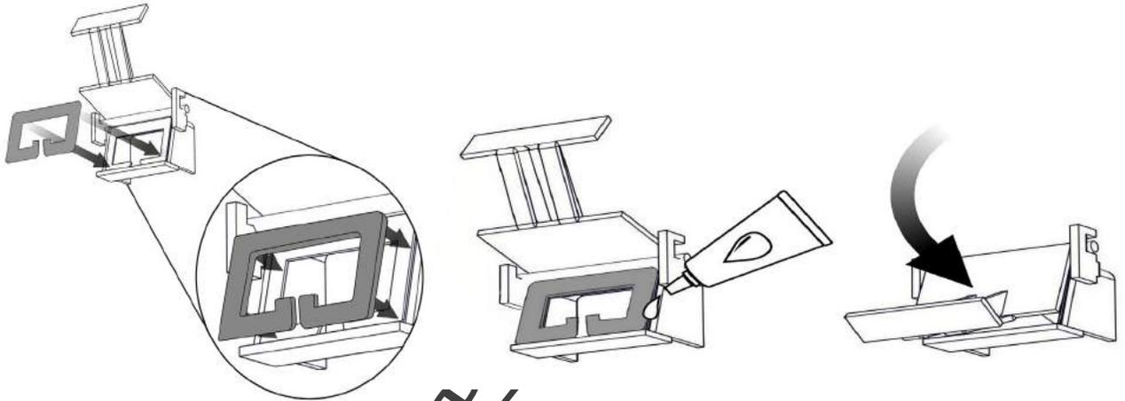
Apply new gasket using stove cement (not supplied) to secure. This is to prevent the ends from fraying and locking the gasket into the position of the gasket groove.
