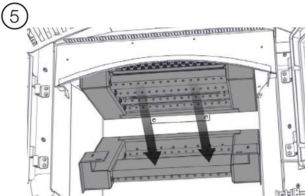
Slide secondary air manifold downward and out to remove. Scrape off gasket from rear and clean surface. Secure new gasket with high temp silicone (not supplied).
