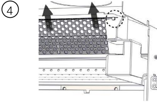
Move perforated catalyst shield up and over shoulder bolts.
