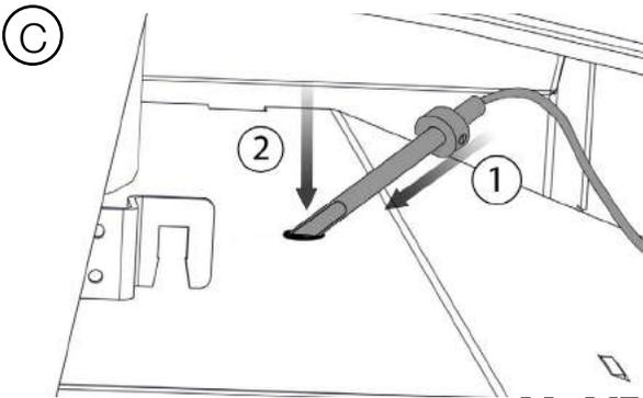
Insert the probe on an angle and gradually straighten the probe so that it aims down.
