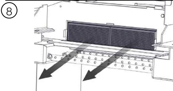
Slide the catalyst forward and out. The steel tabs are friction held and will separate from the catalyst when pulled out.
