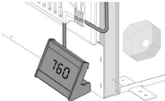
OPTION 2. The bottom trim may be loosely assembled to the appliance to allow a gap for the wire to feed through.
