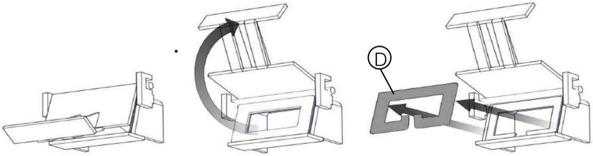
Open dilution door and remove gasket.
