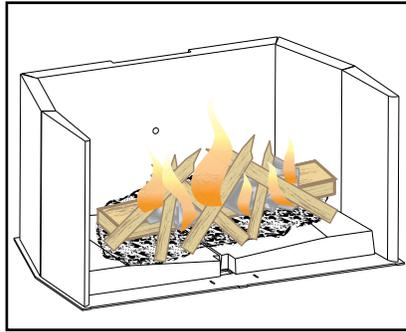
**E.** Slowly add larger wood (2x4 size pieces). Lay the pieces length wise from side to side in the hot coal bed with a shallow trench between, so that the primary air can flow directly into this trench and ignite the fuel above.
