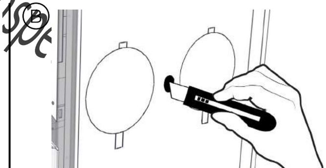
Cut away or poke through the insulation to provide a route for the probe.
