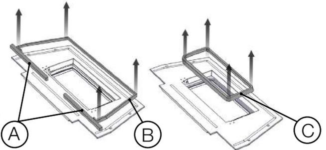
Remove gaskets A,B and C.
