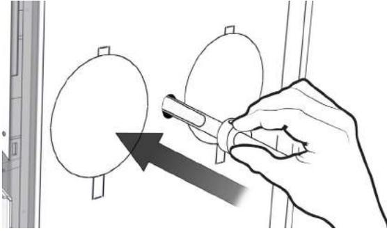
From the outside of the appliance insert the probe rod end through the knockout hole.
