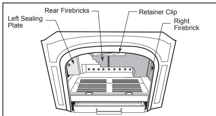
Figure 33 - Remove left and right sealing plates.
