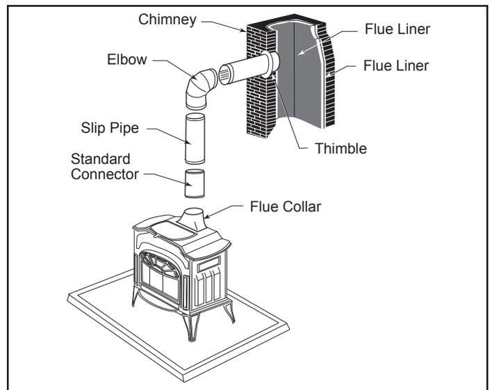
**Figure 6** - Chimney connection is a freestanding installation.
