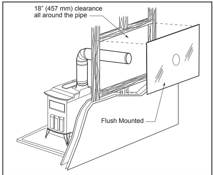
Figure 10 - An approved wall pass-through for Canada.
