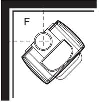
\* This distance, from the center of the flue collar to the front edge of the hearth, is the same for all installations on this page: 35" in the United States and 37" (940mm) in Canada.
