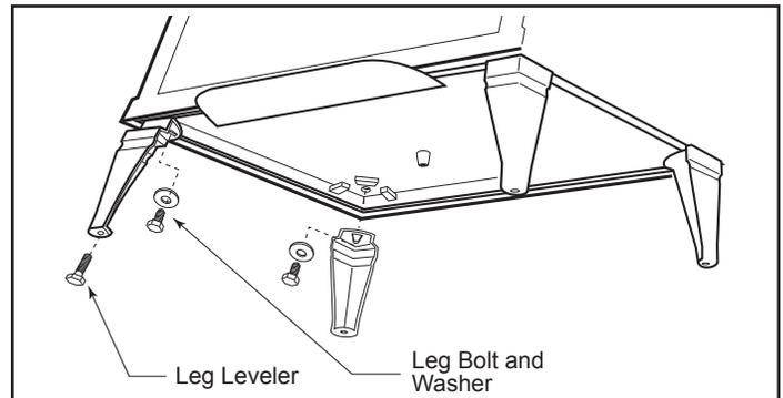
**Figure 26a - Attach stove legs and leg levelers.**
