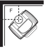
\*\*To locate center of flue collar for corner installation, add 10 1/2" (270mm) to the clearance distance from stove corner to wall. Mark off the resulting distance from the corner along both walls. Next, measure the same distance from these two points out from the walls. These last two measurements will meet at a point representing the center of the flue collar. Refer to the diagrams above.
